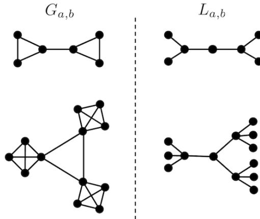
Figure 11: Examples of graphs of the model classes  $G_{a,b}$  and  $L_{a,b}$  (top:  $a = b = 2$ , bottom:  $a = b = 3$ ). For both pairs,  $G_{a,b}$  is the line graph of  $L_{a,b}$ .
